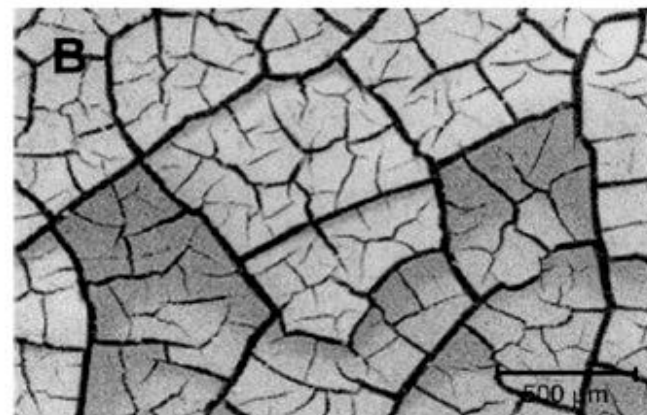
sample surface aged under QUV for 800 h (Küpper, et al., 2004)
